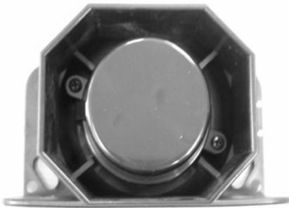
Heavy duty construction 107 dba backup alarms for mobile equipment features multivoltage, weatherproof housing and "AA" self-adjusting sound level = 5db above surrounding noise.
