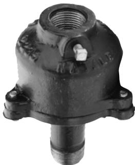
Extend lamp life with this cast aluminum shock mount. The lighting fixture floats on a solid rubber base that absorbs shock and vibration. A ground connection is installed between the top and bottom of the shock mount for added safety.
