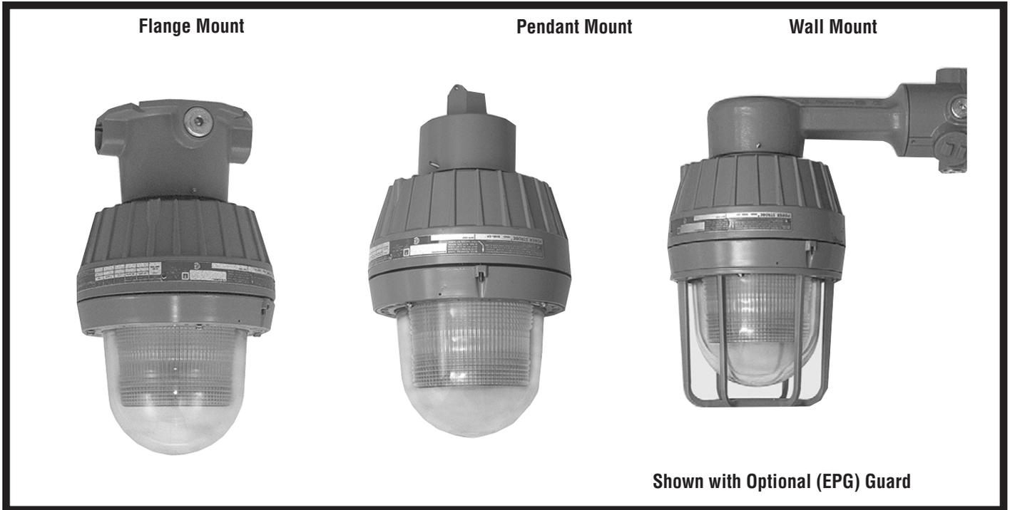
The Super Explosion Proof family of double flash UL listed strobe lights are designed for operation in hazardous areas rated by the NEC as Class I, div 1 & 2 Group C & D and Class II, div. 1 & 2, Group E, F, & G and Class III, div. 1 & 2. They also meet NEMA standards 3, 4, 4X, 7CD and 9EFG, and are marine rated for use in salt water environments. Lens Colors: Amber, Blue, Clear, Green, Purple and Red.
