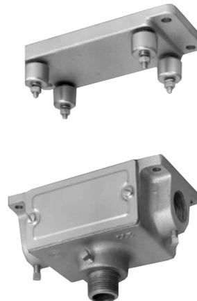
This combination shock mount and junction box protects against shock and vibration while offering the added feature of a junction box. The shock mount must be ordered with the junction box. The junction box can be ordered separately.
