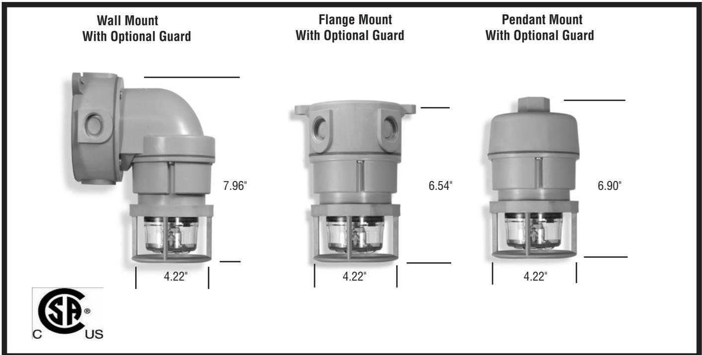
Tomar Electronics introduces the Model 2000XL family of Hazardous Location Div. 2 LED Lights engineered to perform in the harshest environments. Constructed of 30% glass-filled thermoset polyester, it is particularly well suited for installations in corrosive, wet NEMA 4X harsh environments, and hazardous locations. The high strength FRP material is resistant to the corrosive effects of most chemicals, hydrocarbons and solvents.
