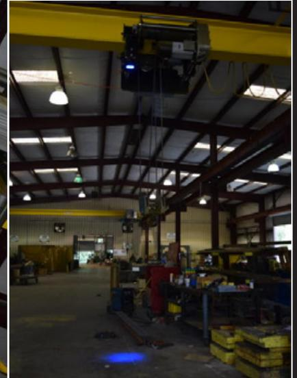
A LED safety spot light, designed to project a bright Blue/Red(or other colors) beam pattern on the ground and serve as a visual warning indicator. It projects a sizeable and powerful beam pattern, ideal for applications such as cranes or other tall equipment where the light needs to travel a further distance without sacrificing on intensity.
