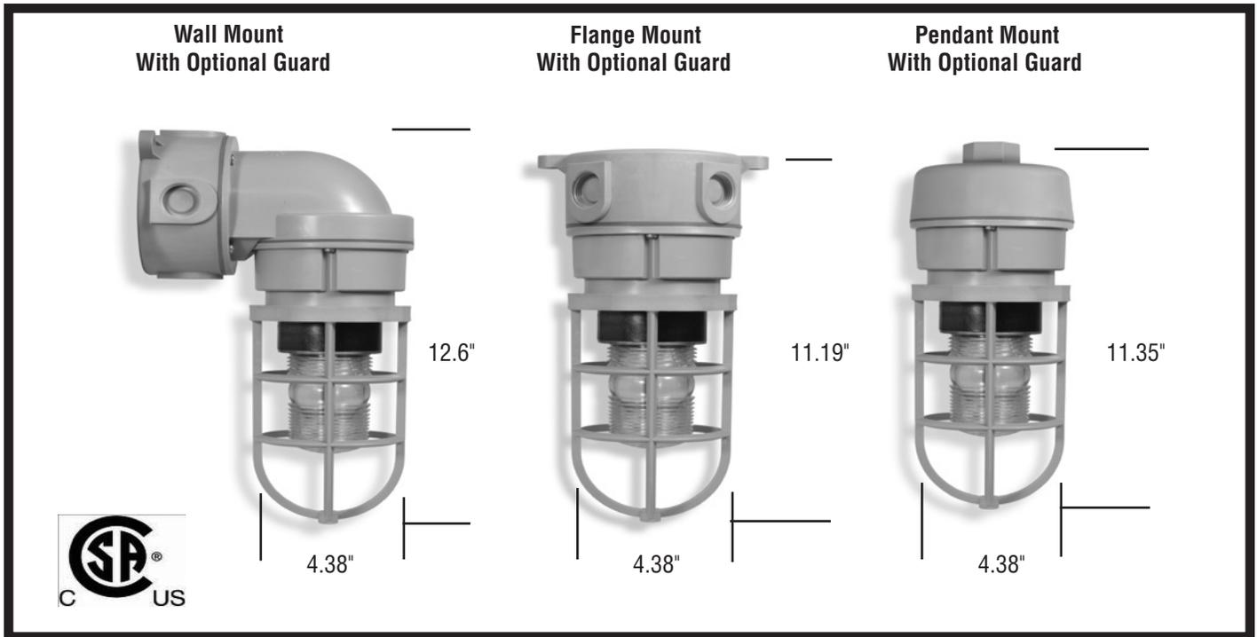
Tomar Electronics introduces the Model 4000X family of Hazardous Location Div. 2 Strobe Lights engineered to perform in the harshest environments. Constructed of 30% glass-filled thermo-set polyester, it is particularly well suited for installations in corrosive, wet NEMA 4X harsh environments, and hazardous locations. The high strength FRP material is resistant to the corrosive effects of most chemicals, hydrocarbons and solvents.
