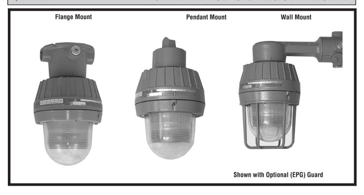
The Super Explosion Proof family of double flash UL listed strobe lights are designed for operation in hazardous areas rated by the NEC as Class I, div 1 & 2 Group C & D and Class II, div. 1 & 2, Group E, F, & G and Class III, div. 1 & 2. They also meet NEMA standards 3, 4, 4X, 7CD and 9EFG, and are marine rated for use in salt water environments. Lens Colors: Amber, Blue, Clear, Green, Purple and Red.
