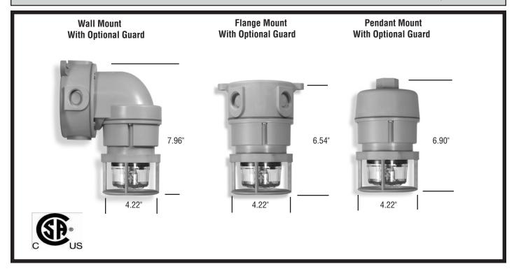
Tomar Electronics introduces the Model 2000XL family of Hazardous Location Div. 2 LED Lights engineered to perform in the harshest environments. Constructed of 30% glass-filled thermoset polyester, it is particulary well suited for installations in corrosive, wet NEMA 4X harsh environments, and hazardous locations. The high strength FRP material is resistant to the corrosive effects of most chemicals, hydrocarbons and solvents.
