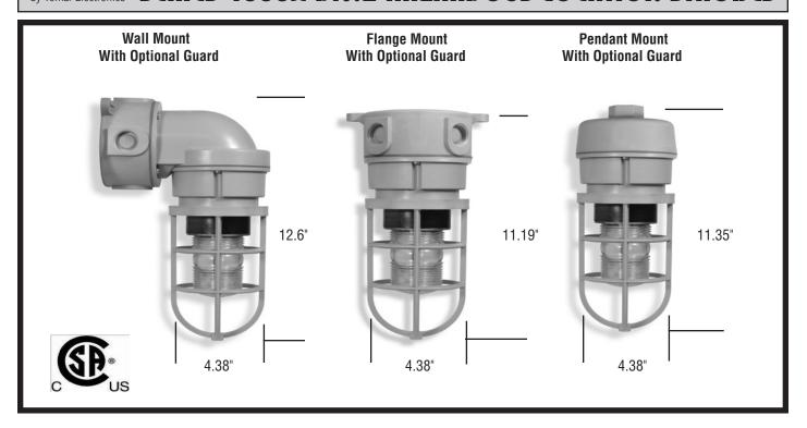
Tomar Electronics introduces the Model 4000X family of Hazardous Location Div. 2 Strobe Lights engineered to perform in the harshest environments. Constructed of 30% glass-filled thermoset polyester, it is particulary well suited for installations in corrosive, wet NEMA 4X harsh environments, and hazardous locations. The high strength FRP material is resistant to the corrosive effects of most chemicals, hydrocarbons and solvents.
