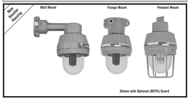
These models of single flash explosion proof UL listed strobe lights are designed for operation in hazardous areas rated Class I DIV. 1 & 2, Group C & D and Class II DIV. 1 & 2, group E, F, & G, & Class III Div. 1 & 2. Design features include a housing made of die cast high strength copper-free aluminum alloy with baked powder epoxy finish, stainless
